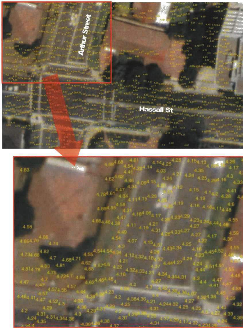
■ Figure A-1: Sample of airborne laser survey data
