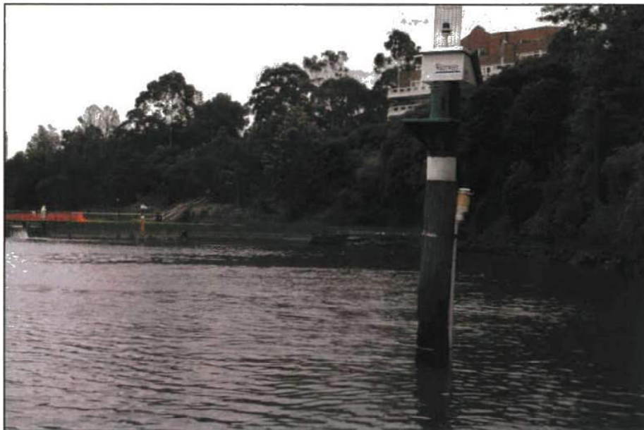
■ Figure 2-2 Tide gauge at Carlingford Railway
