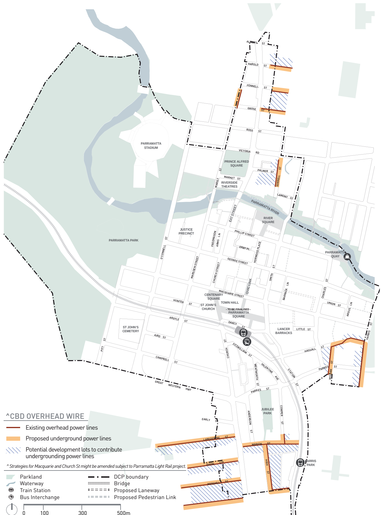
Figure 4.7 CBD - Undergrounding Overhead Wire Strategy
