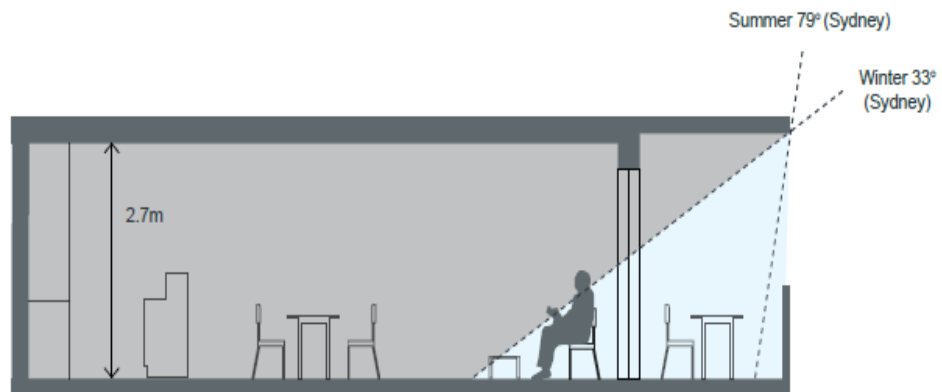
Figure 3.27 Shading devices on balconies should shade summer sun and allow winter sun access to living areas Source: Apartment Design Guide, NSW Department of Planning & Environment
