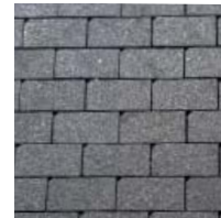
Footpath Material: granite Product: "Adelaide Black (Veined)" or "Austral Black" Size: 200x100x50mm Finish: exfoliated
