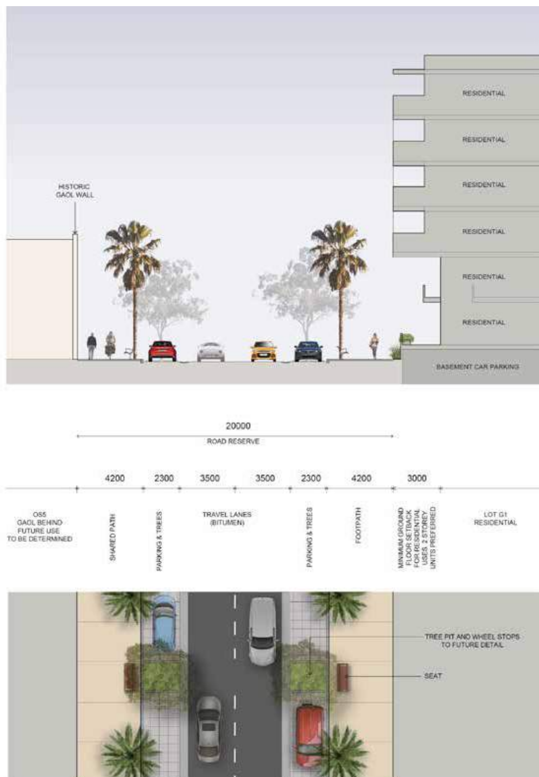
Figure 4.3.6.8 Typical street section 3 – Dunlop Street
