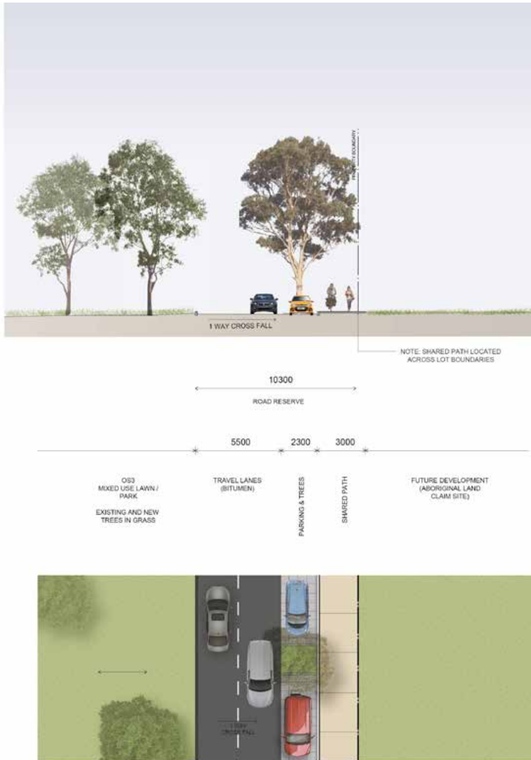
Figure 4.3.6.13 Typical street section 8 – East Circuit (north)
