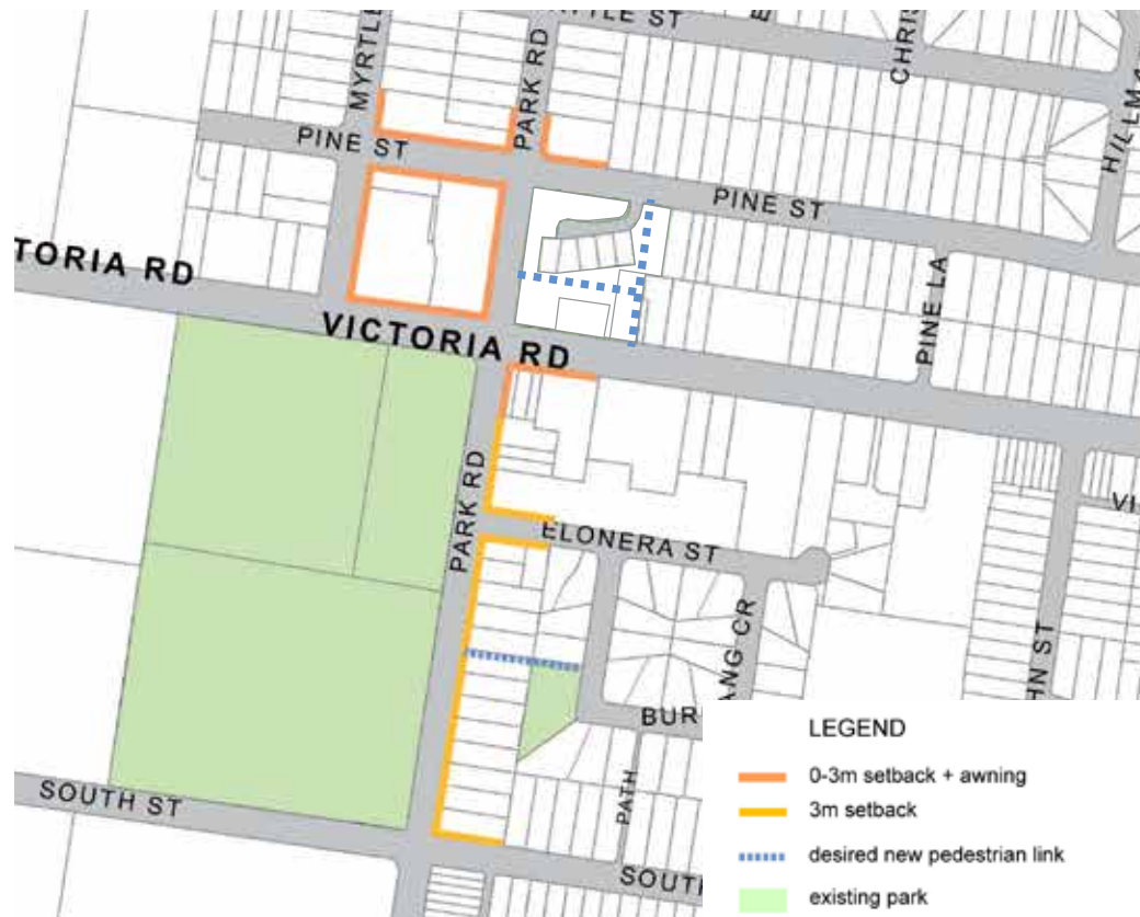
Figure 4.1.4.2 Building Setbacks and Pedestrian Links
