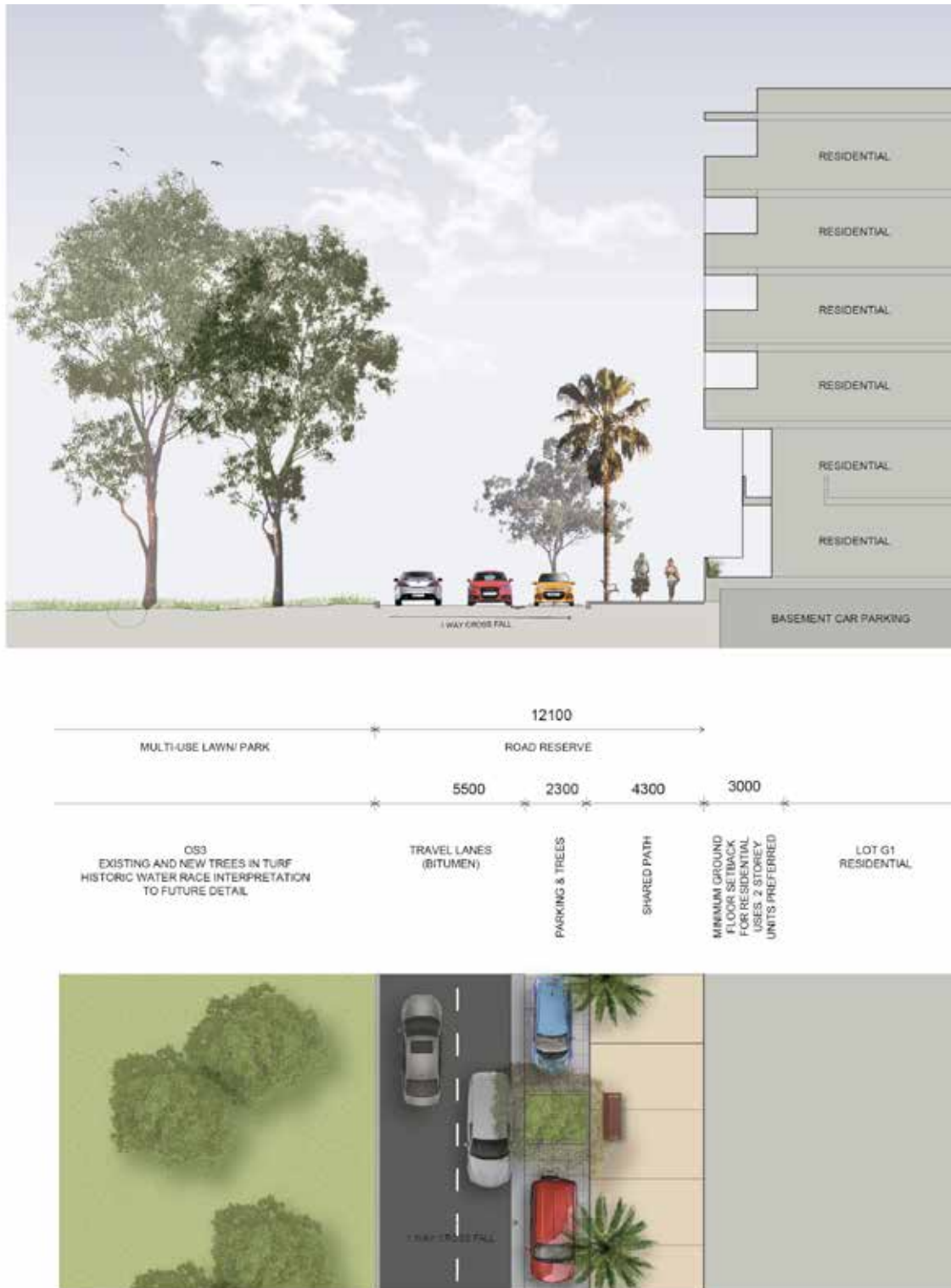
Figure 4.3.6.11 Typical street section 6 – East Circuit (east)
