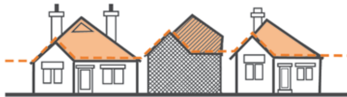
Figure 3.2.3.1 Sympathetic and complementary roof designs
