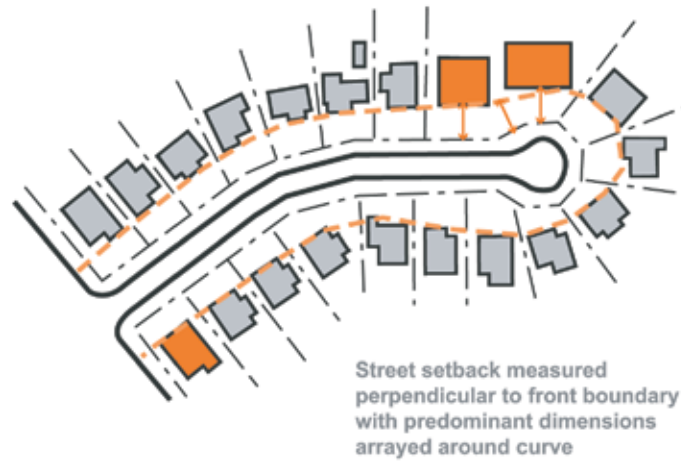
Figure 3.2.5.3 Building frontage setbacks - curvilinear street
