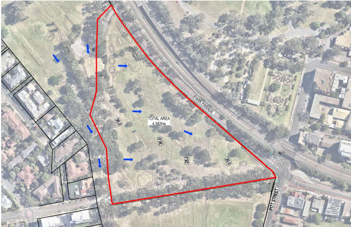
Figure 3 – Existing Topography and Catchments
