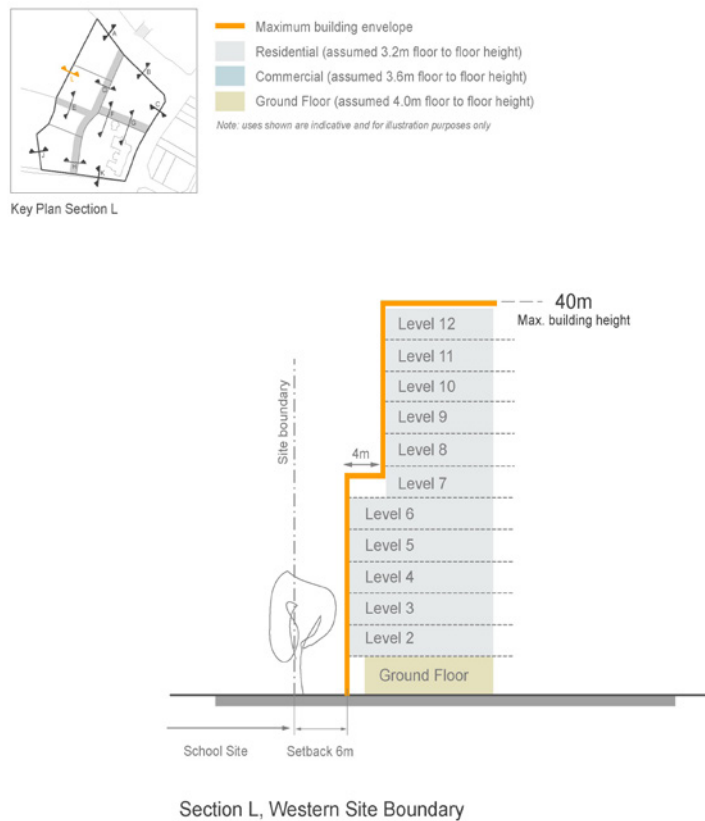
Figure 4.3.4.1.15 Indicative Site Sections
