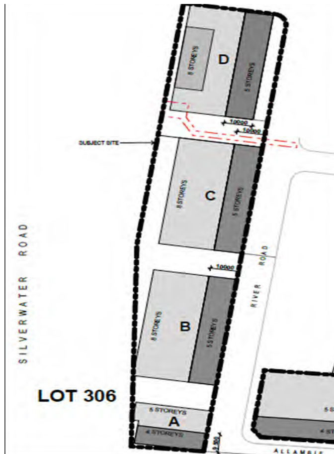
Figure 4.3.5.5 Setback of building height for Lot 306
