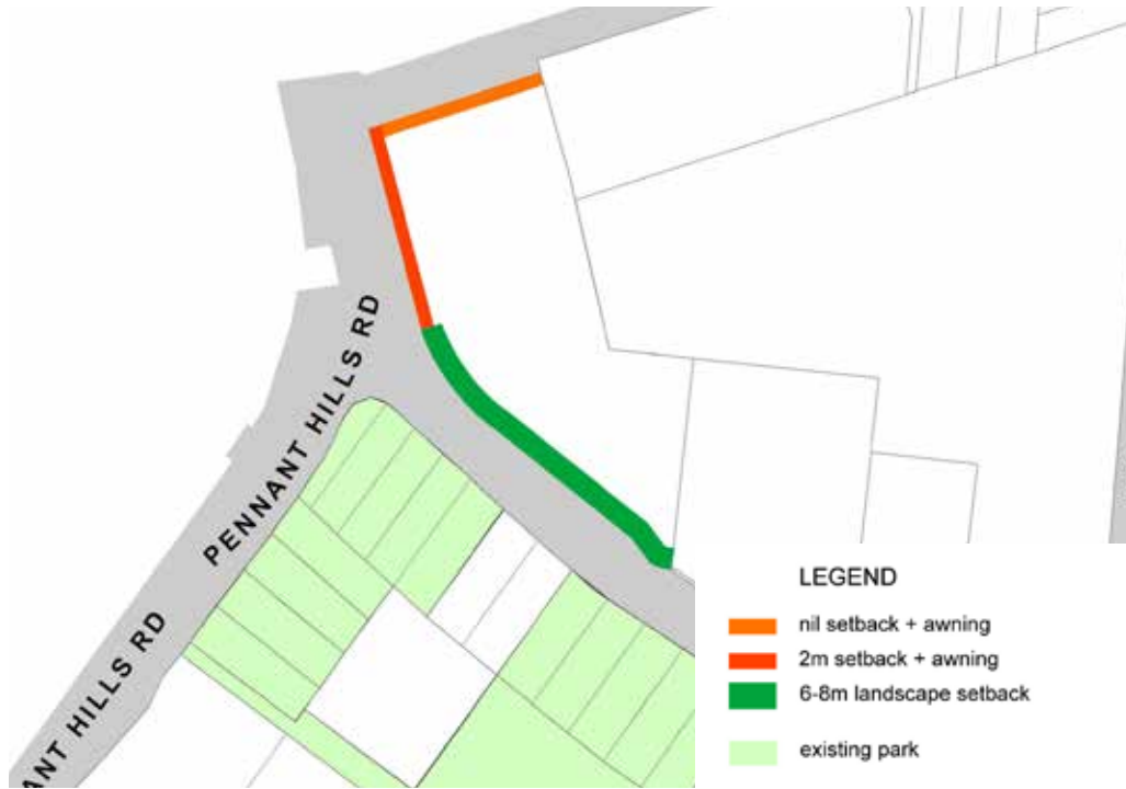
Figure 4.1.1.4 Ground Level Setbacks
