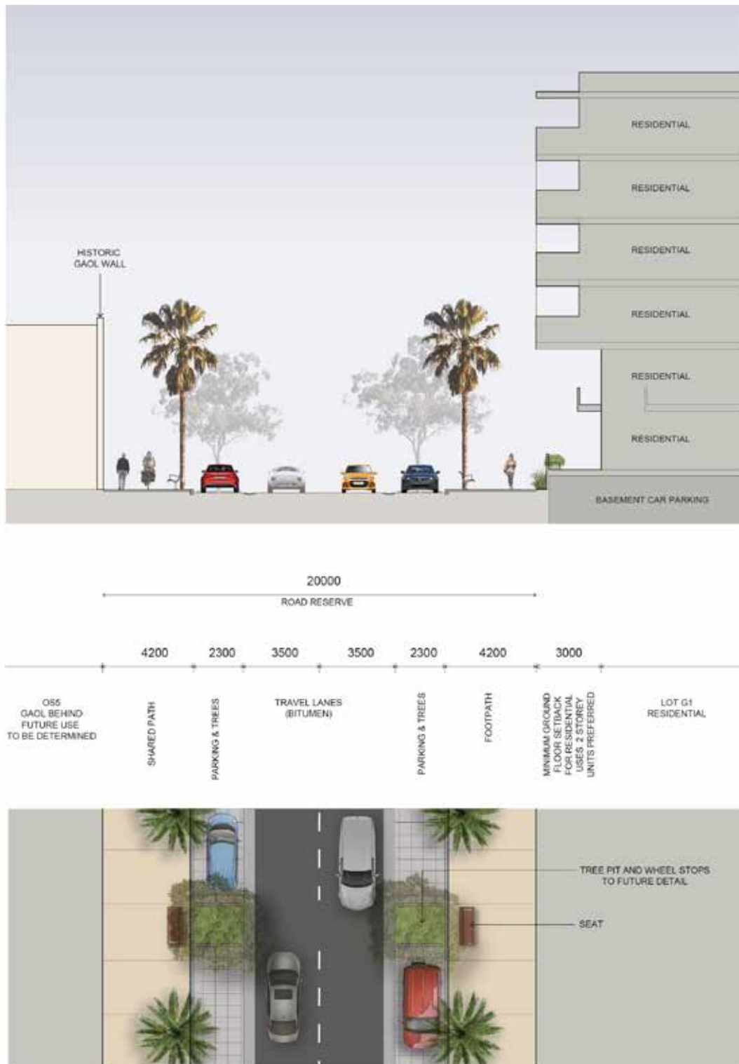
Figure 4.3.6.8 Typical street section 3 – Dunlop Street
