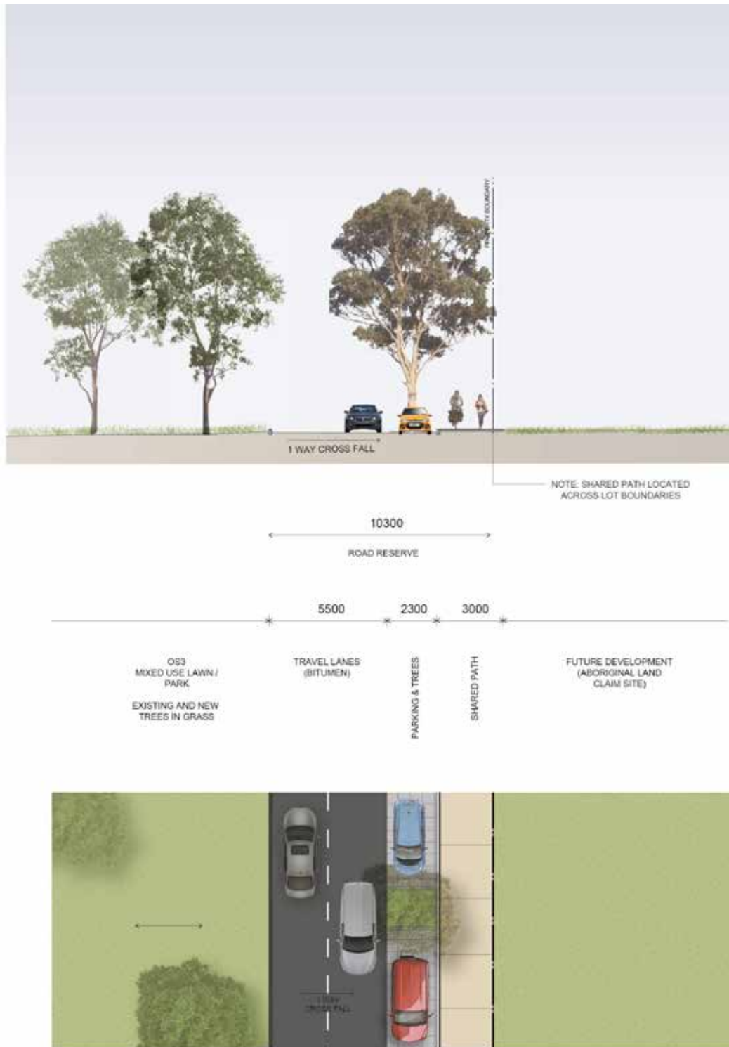
Figure 4.3.6.13 Typical street section 8 – East Circuit (north)
