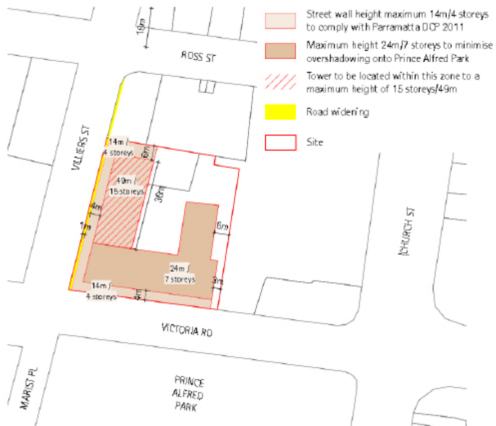
Figure 4.3.3.7.22 Built Form Design Controls – Heights and Setbacks
