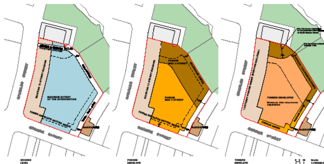
Figure 4.3.3.7.26 Building heights, setbacks and envelopes
