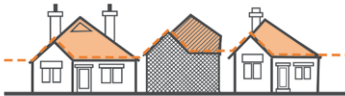
Figure 3.2.3.1 Sympathetic and complementary roof designs
