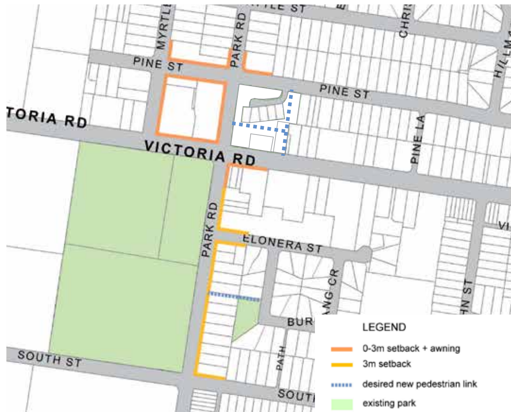
Figure 4.1.4.2 Building Setbacks and Pedestrian Links
