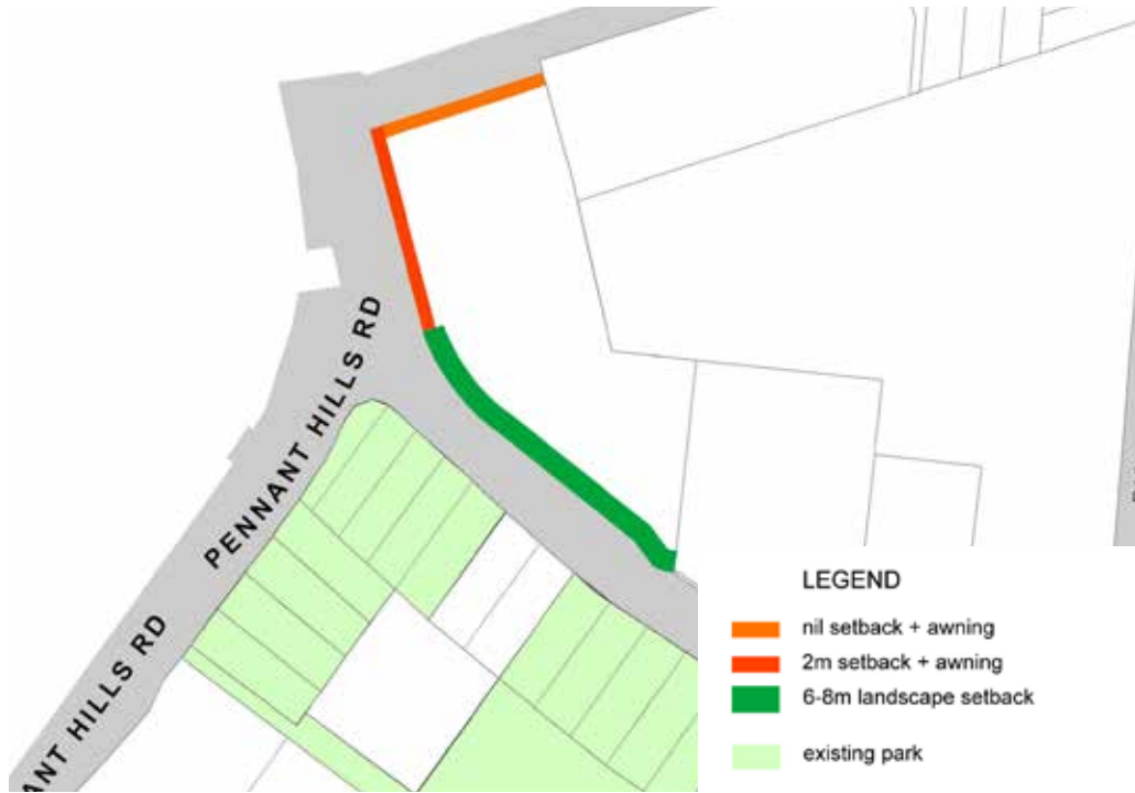
Figure 4.1.1.4 Ground Level Setbacks
