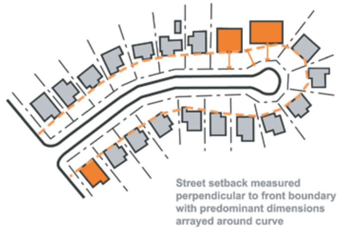
Figure 3.2.5.3 Building frontage setbacks - curvilinear street
