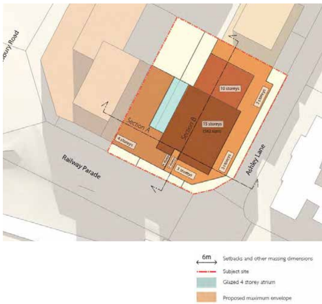
Figure 4.3.4.2.2 Built form design controls - Storeys
