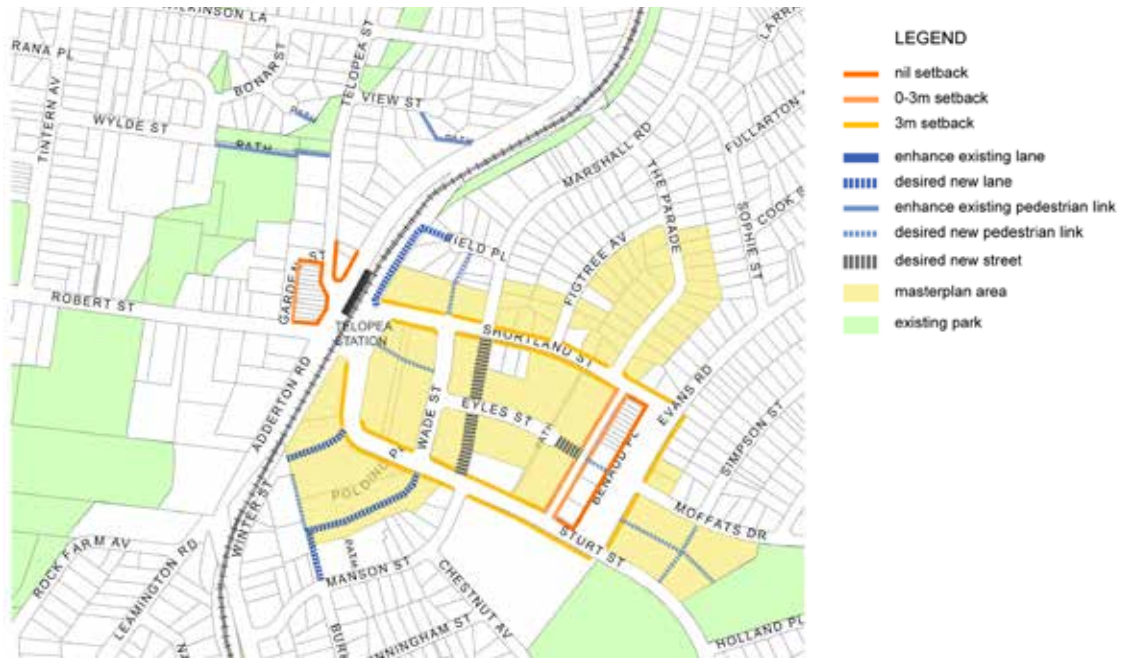
Figure 4.1.11.2 Building Setbacks, Laneways and pedestrian links
