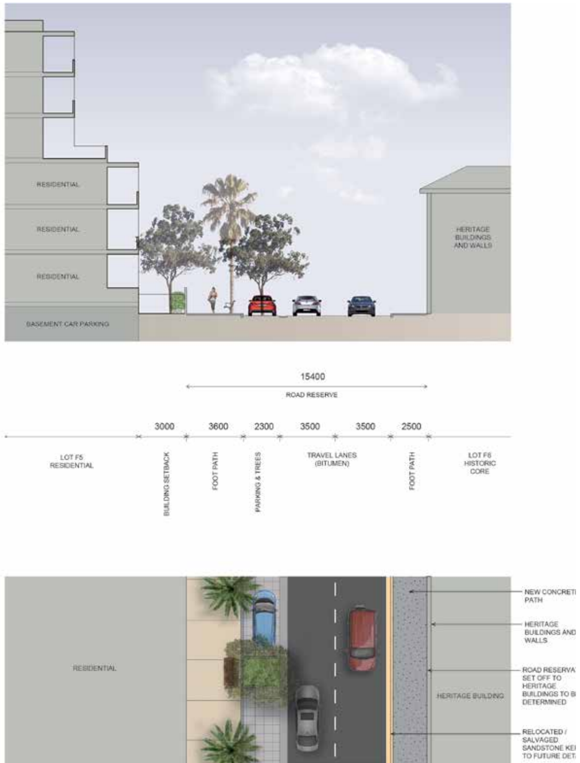
Figure 4.3.6.9 Typical street section 4 – River Road
