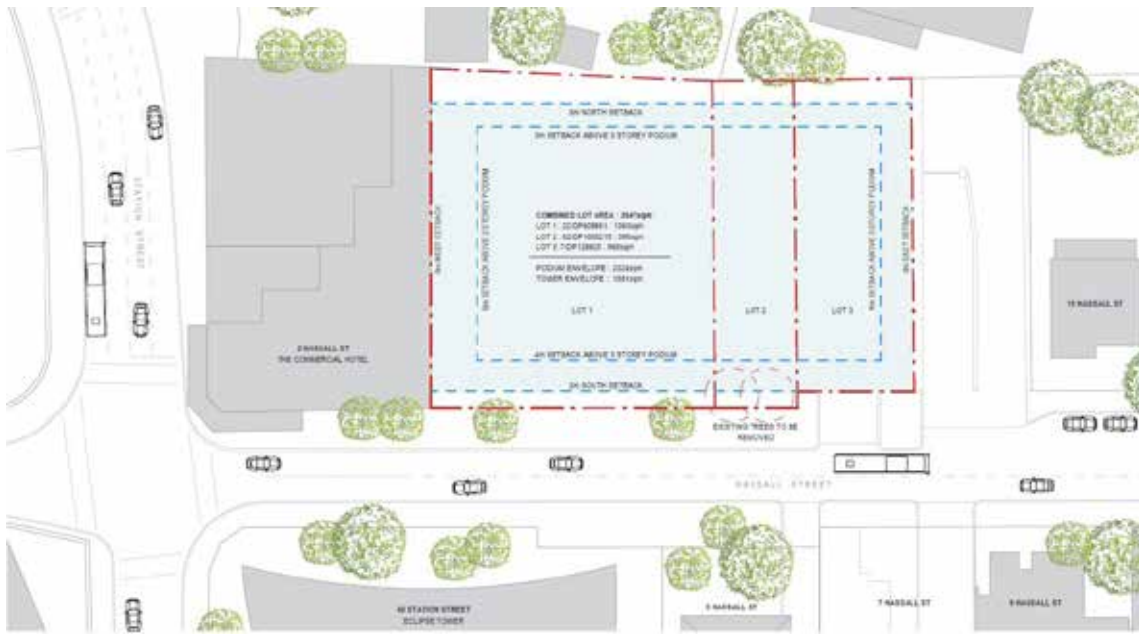
Figure 4.3.3.7.43 Building Setback Control
