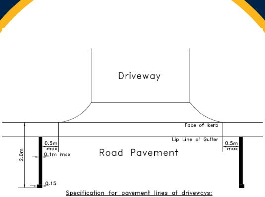
Lines to be marked by an appropriate contractor in a workman like manner, using white paint, in accordance with the above dimensions.
