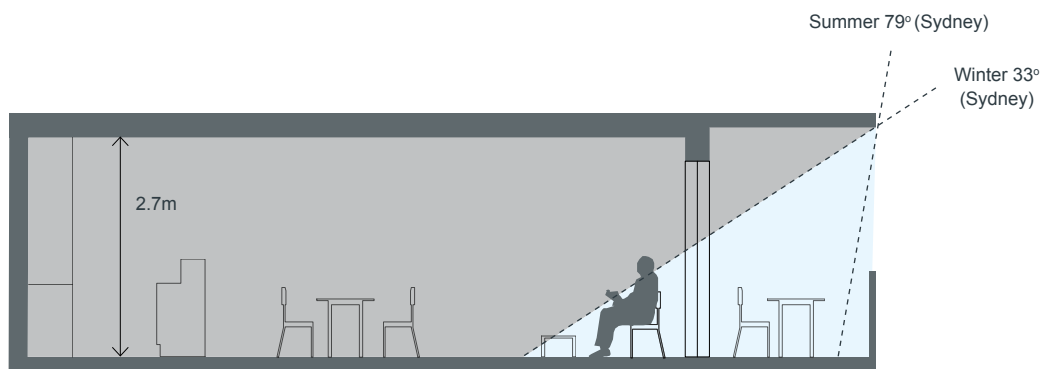
Figure 3.3.5.4 Shading Devices on balconies should shade summer sun and allow winter sun access to living areas Source: Apartment Design Guide, NSW Department of Planning and Environment
