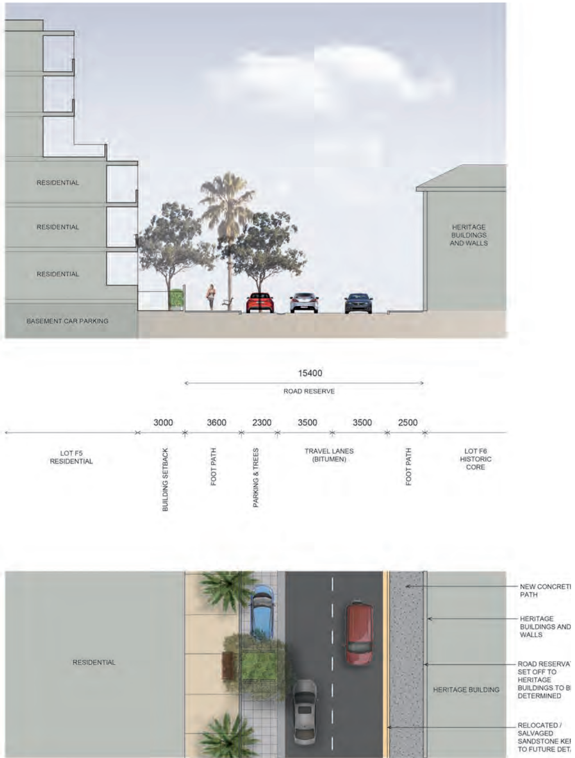
Figure 4.3.6.9 Typical street section 4 – River Road
