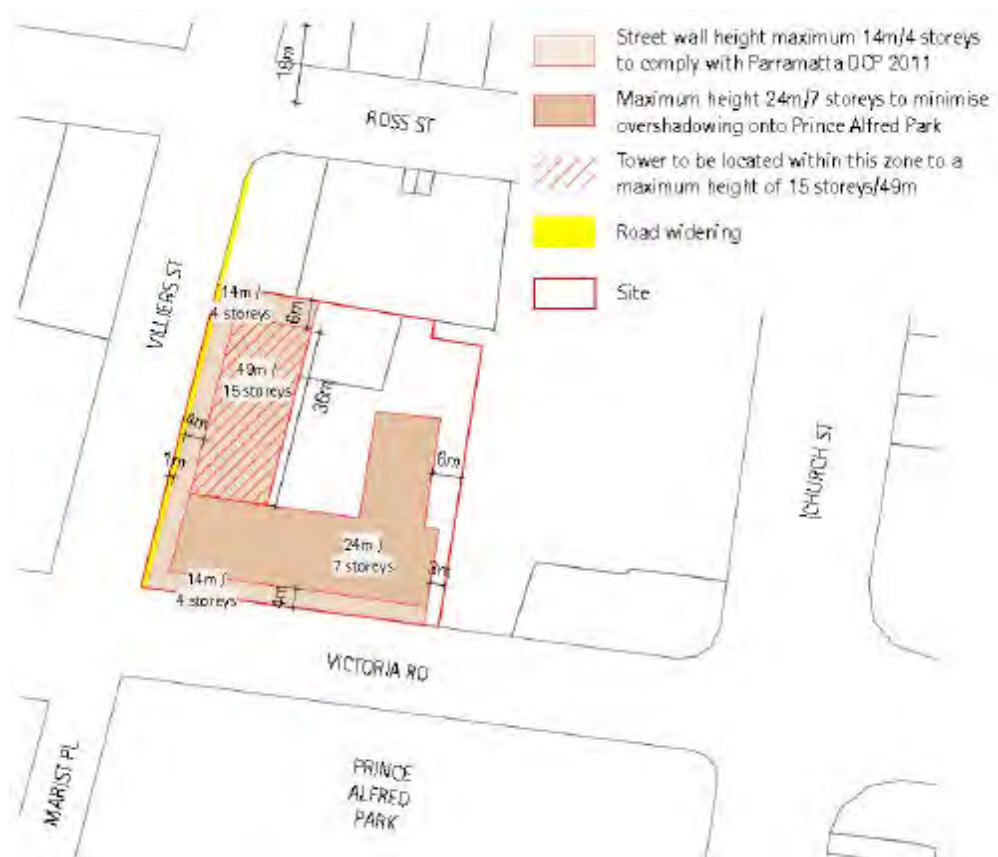
Figure 4.3.3.7.22 Built Form Design Controls – Heights and Setbacks
