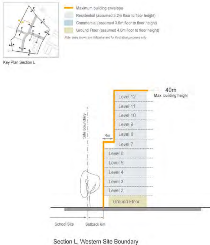
Figure 4.3.4.1.15 Indicative Site Sections
