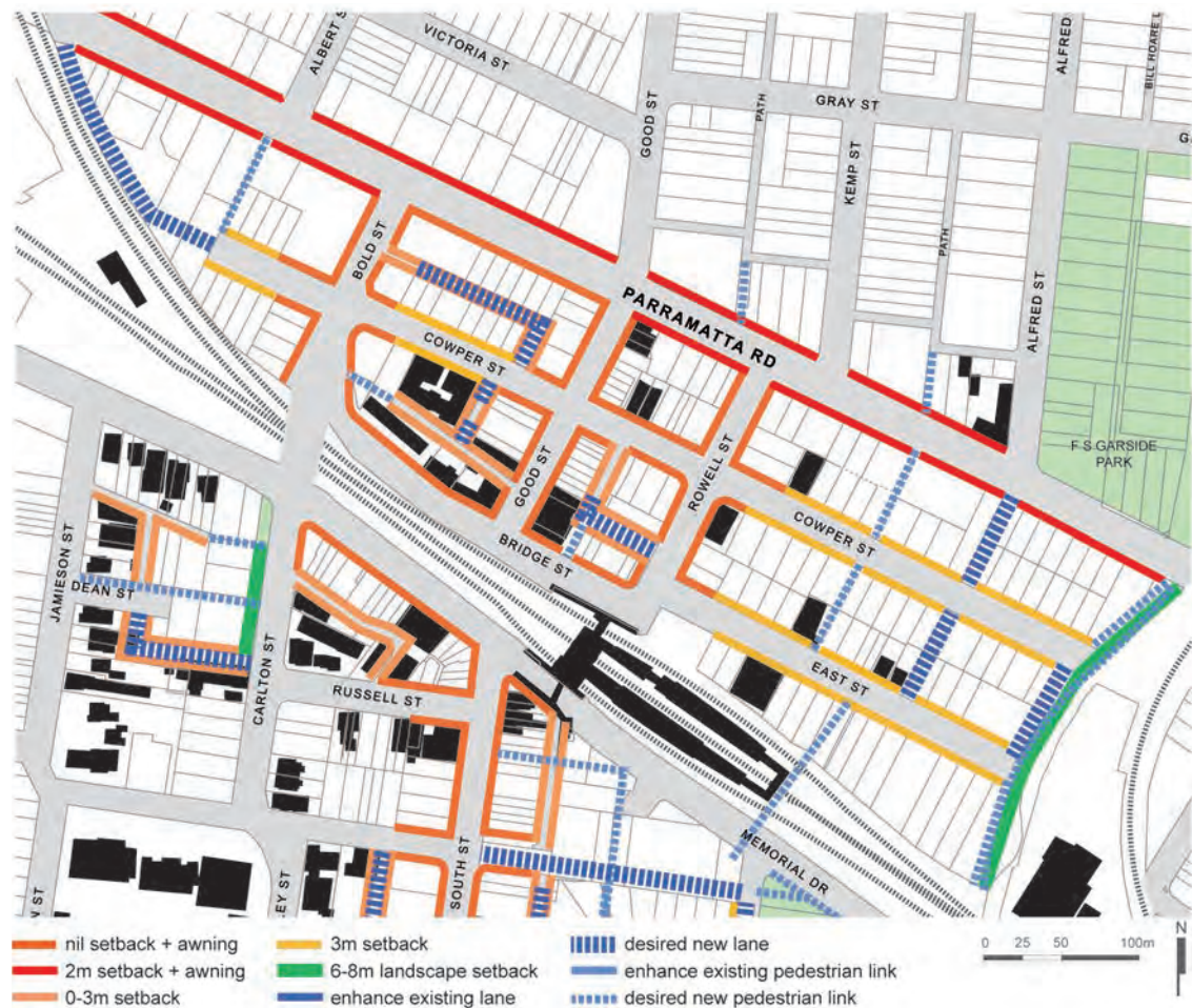
Figure 4.1.6.3 Building Setbacks, Pedestrian Links and Laneways
