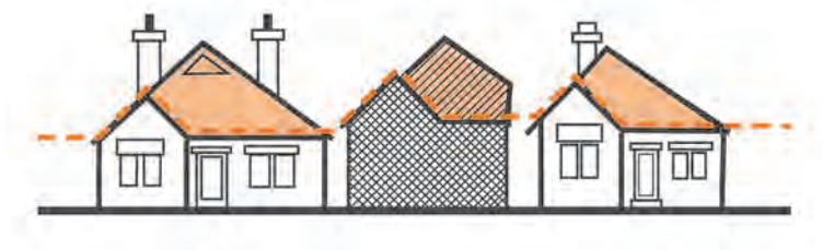
Figure 3.2.3.1 Sympathetic and complementary roof designs
