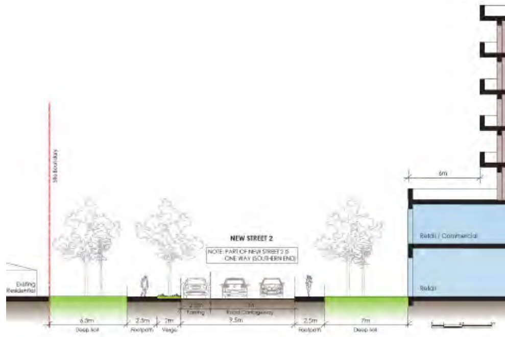
Figure 4.1.12.13 New Street 2 Setbacks – Northern End (Section E-E)
