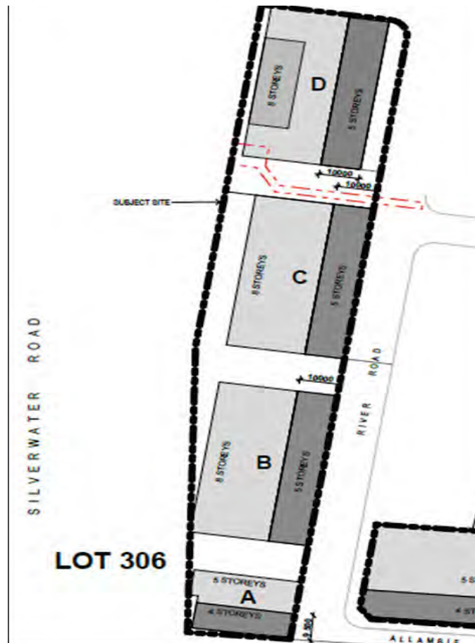
Figure 4.3.5.5 Setback of building height for Lot 306
