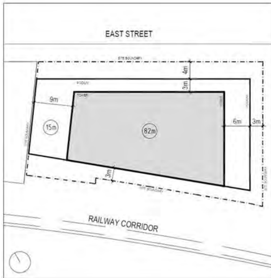
Figure 4.3.7.2.3 Building Height and Setback Control
