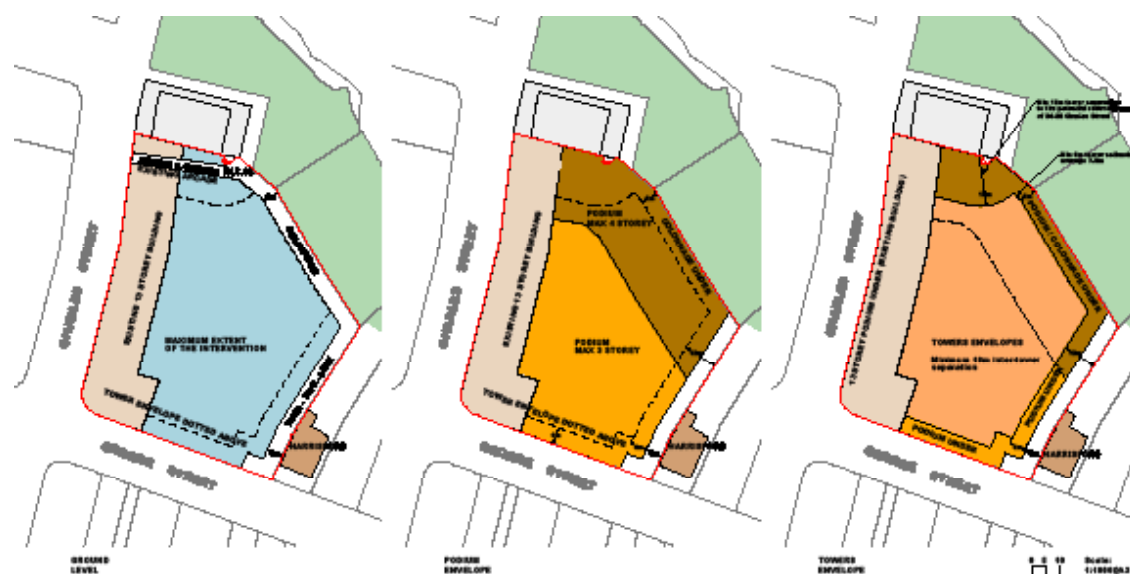
Figure 4.3.3.7.26 Building heights, setbacks and envelopes
