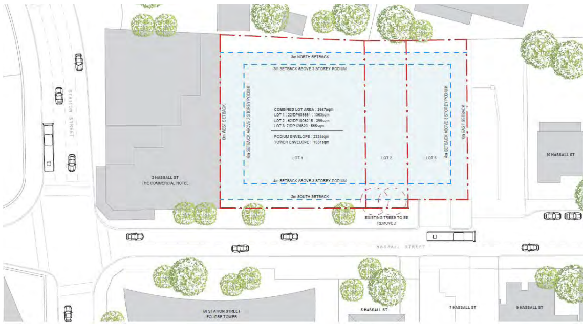
Figure 4.3.3.7.43 Building Setback Control
