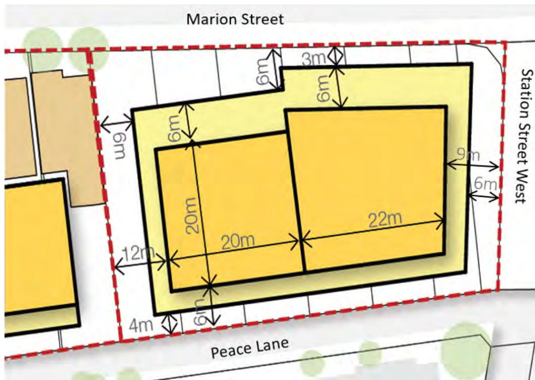
Figure 4.3.3.7.70 Building alignment and setbacks
