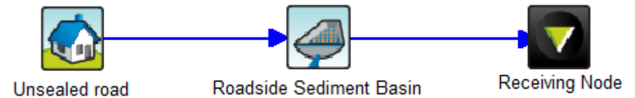
Figure 6-15 Example of Sedimentation Basin Node Application
