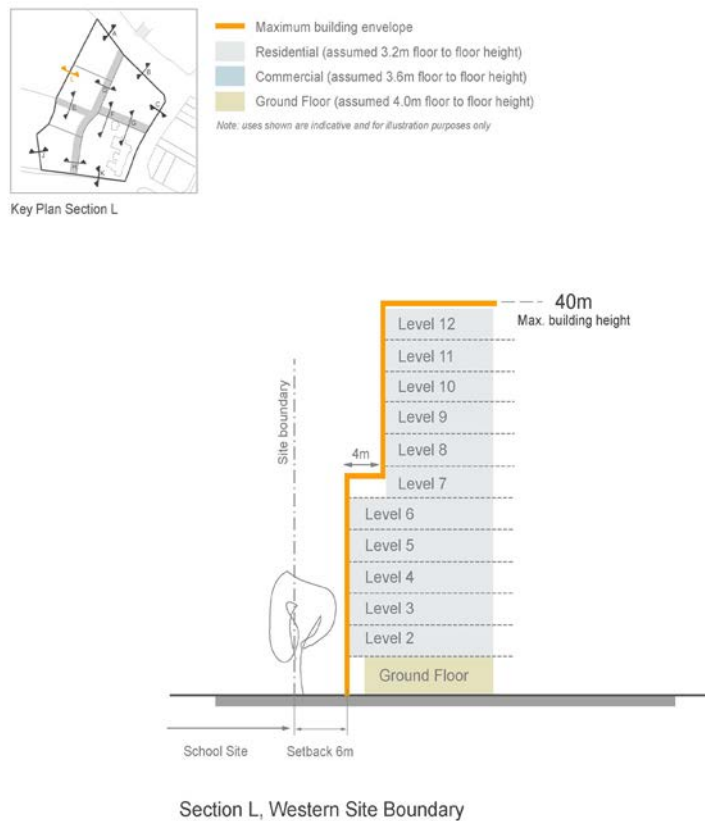
Figure 4.3.4.1.15 Indicative Site Sections
