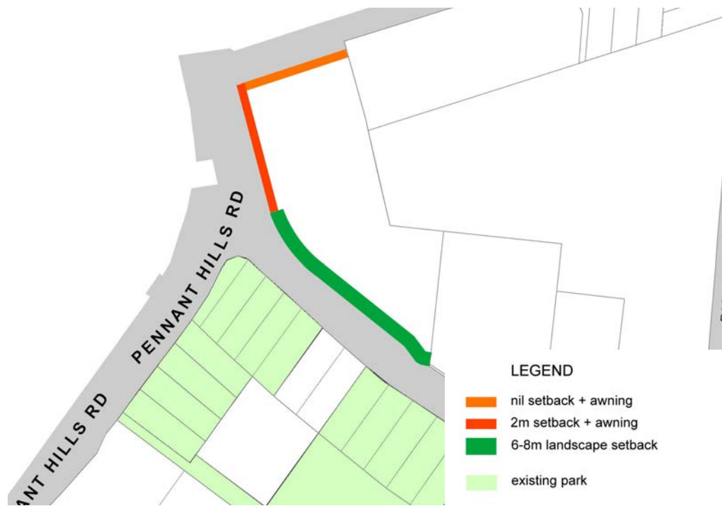
Figure 4.1.1.4 Ground Level Setbacks
