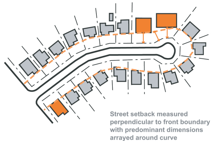
Figure 3.2.5.3 Building frontage setbacks - curvilinear street
