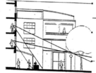
The location of living spaces and position of windows should maximise potential for casual surveillance of streets and public spaces.
