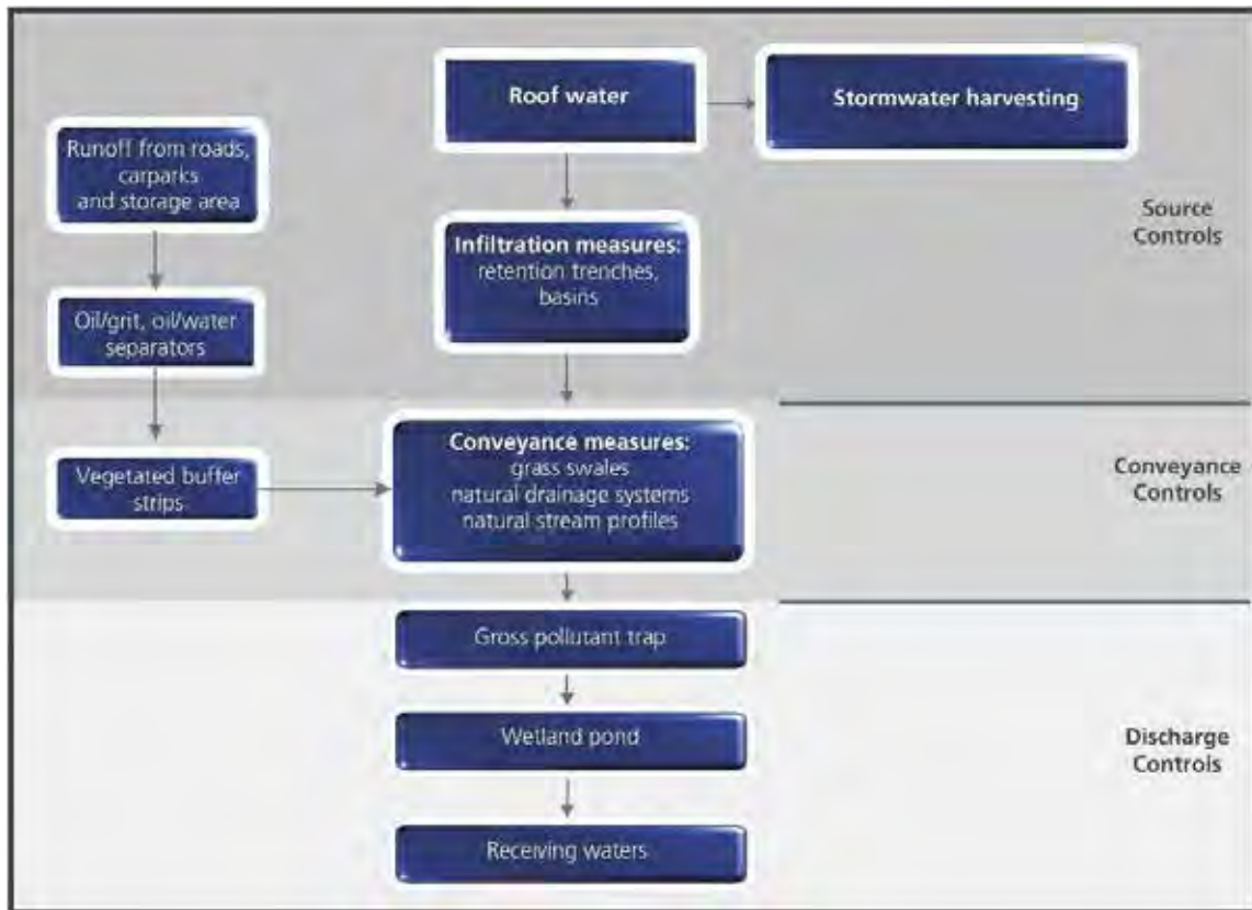
Figure 11: Stormwater Management System
