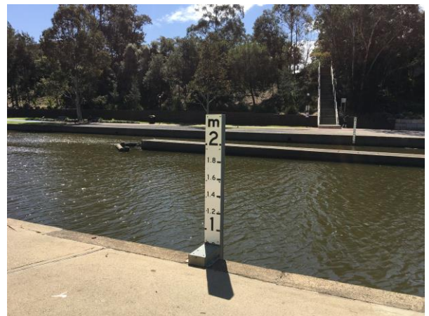
Figure 1-42 Water level gauge at Charles St Weir
