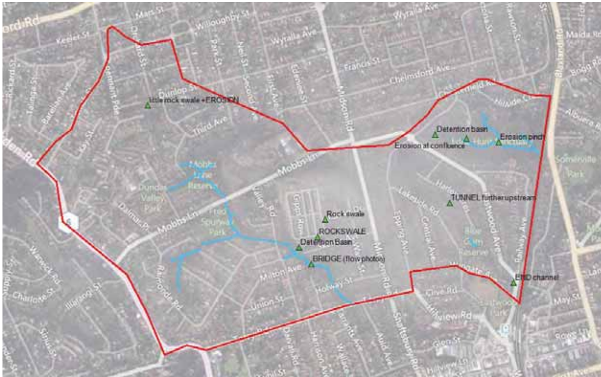
Figure 30 Stormwater treatment and management devices and structures in Terry's Creek Catchment
