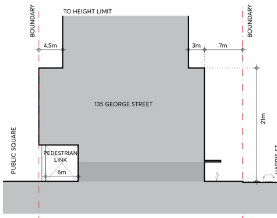
Figure 6.10.10.7 – Section showing double height colonnade and setbacks to tower at the corner of Harris and George Streets
