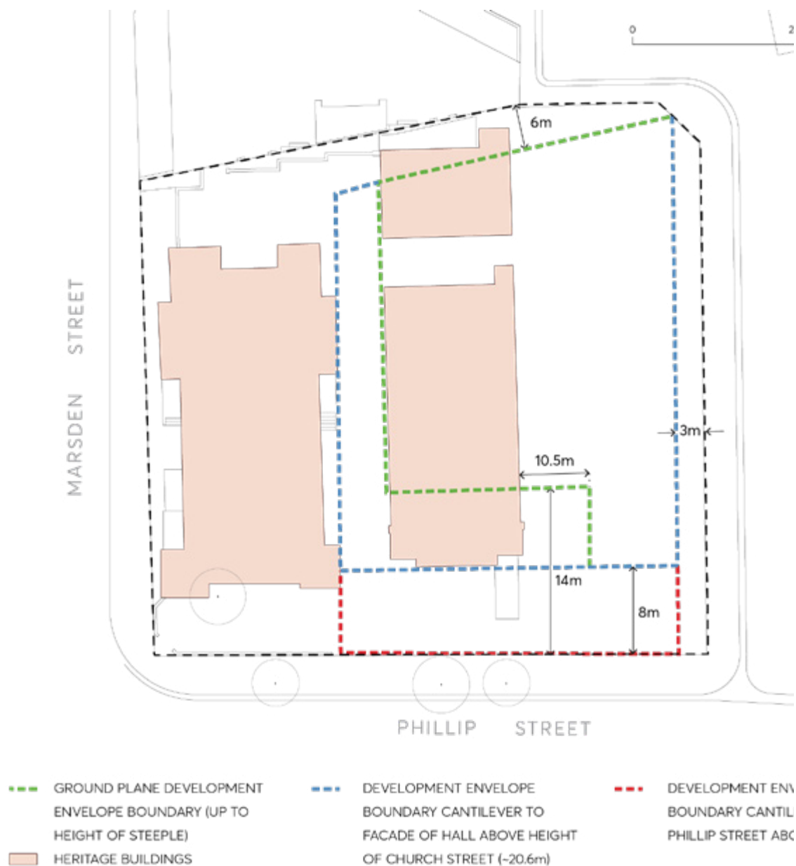
Figure 6.10.4.3 – Existing ground floor plans with building guidelines (Source: TKD Architects)
