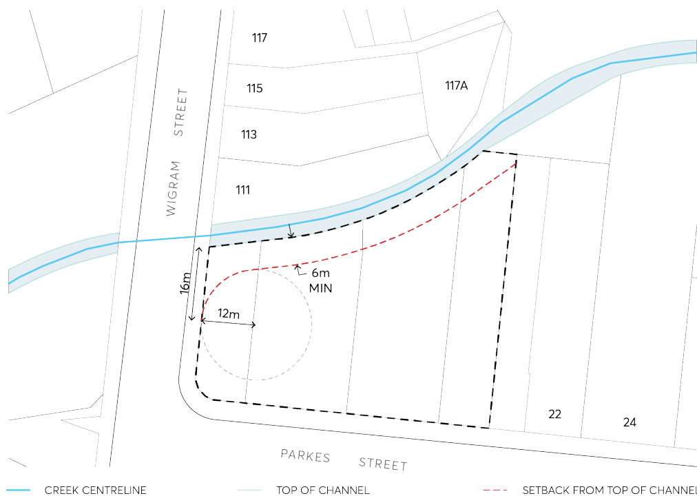
Figure 9.10.8.2 – Required floodway setbacks
