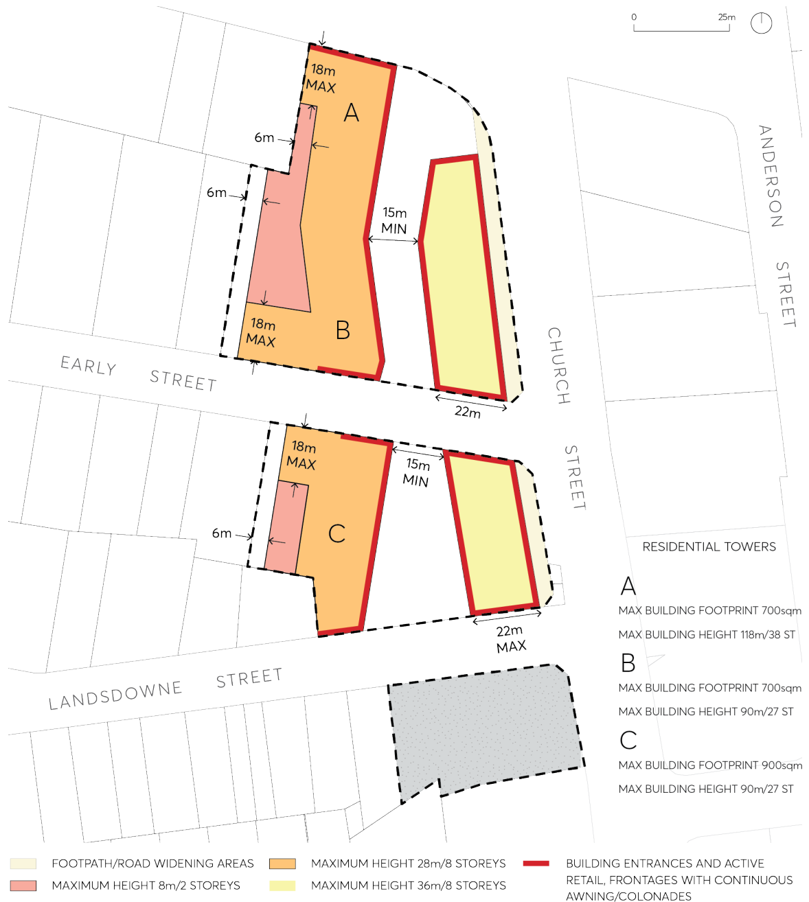
Figure 9.10.2.3 – Building Form Control Plan
