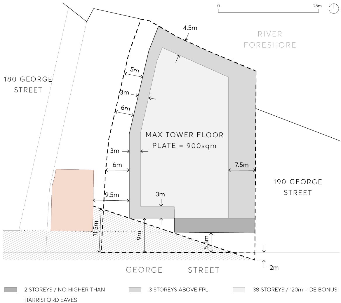
Figure 9.10.5.3 – Setbacks for tower and podium
