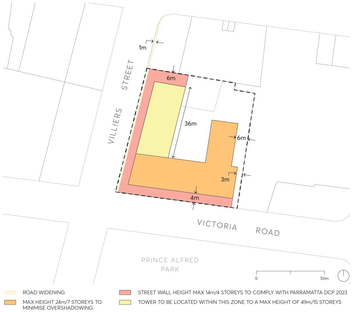
Figure 9.10.19.1 – Built Form Design Controls – Heights and Setbacks
