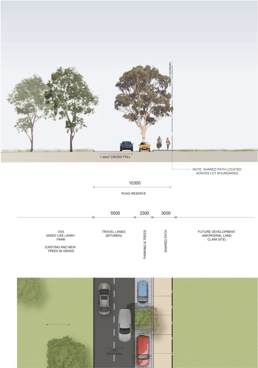
Figure 8.2.2.6.8 - Typical street section 8 – East Circuit (north)
