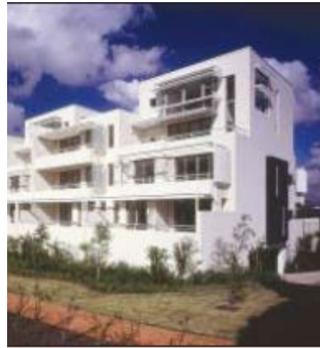
Figure 8.2.8.1.10.2 – Articulate built form to allow daylight access to habitable rooms (Source: Residential Flat Design Code )
