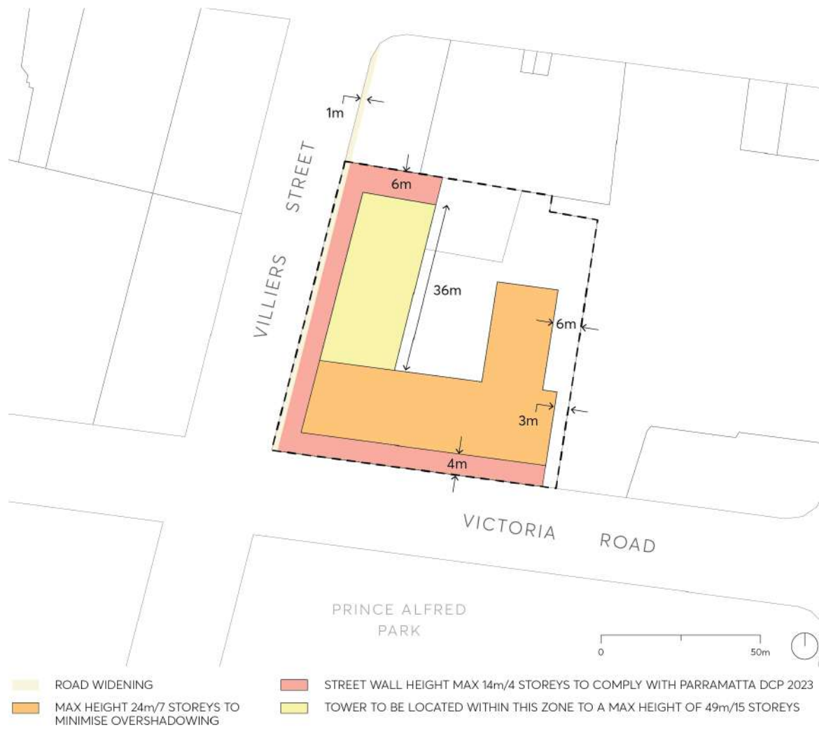
Figure 9.10.19.1 – Built Form Design Controls – Heights and Setbacks
