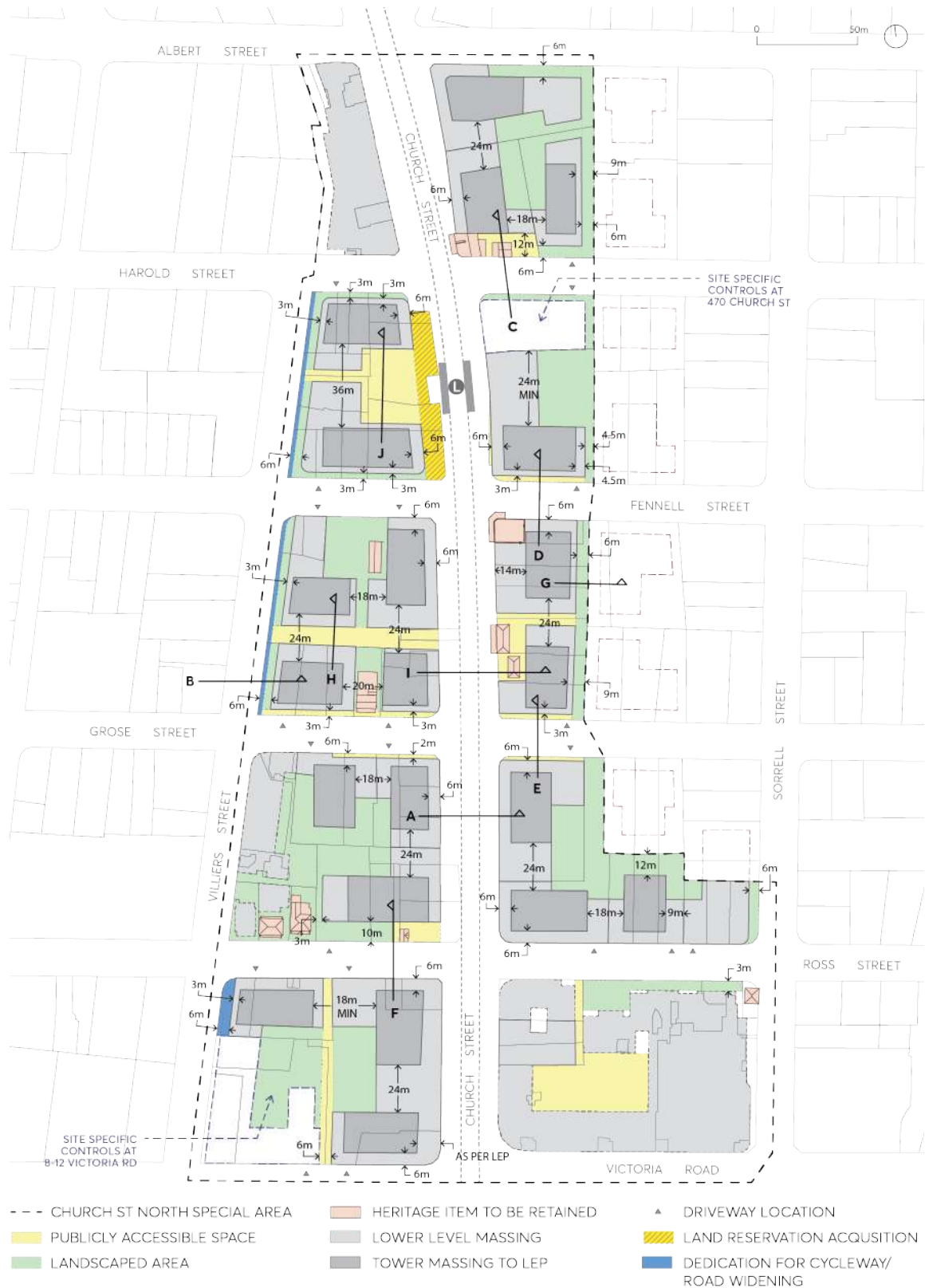
Figure 9.5.11.4 – Church Street North Special Area Required Setbacks &amp; Built Form
