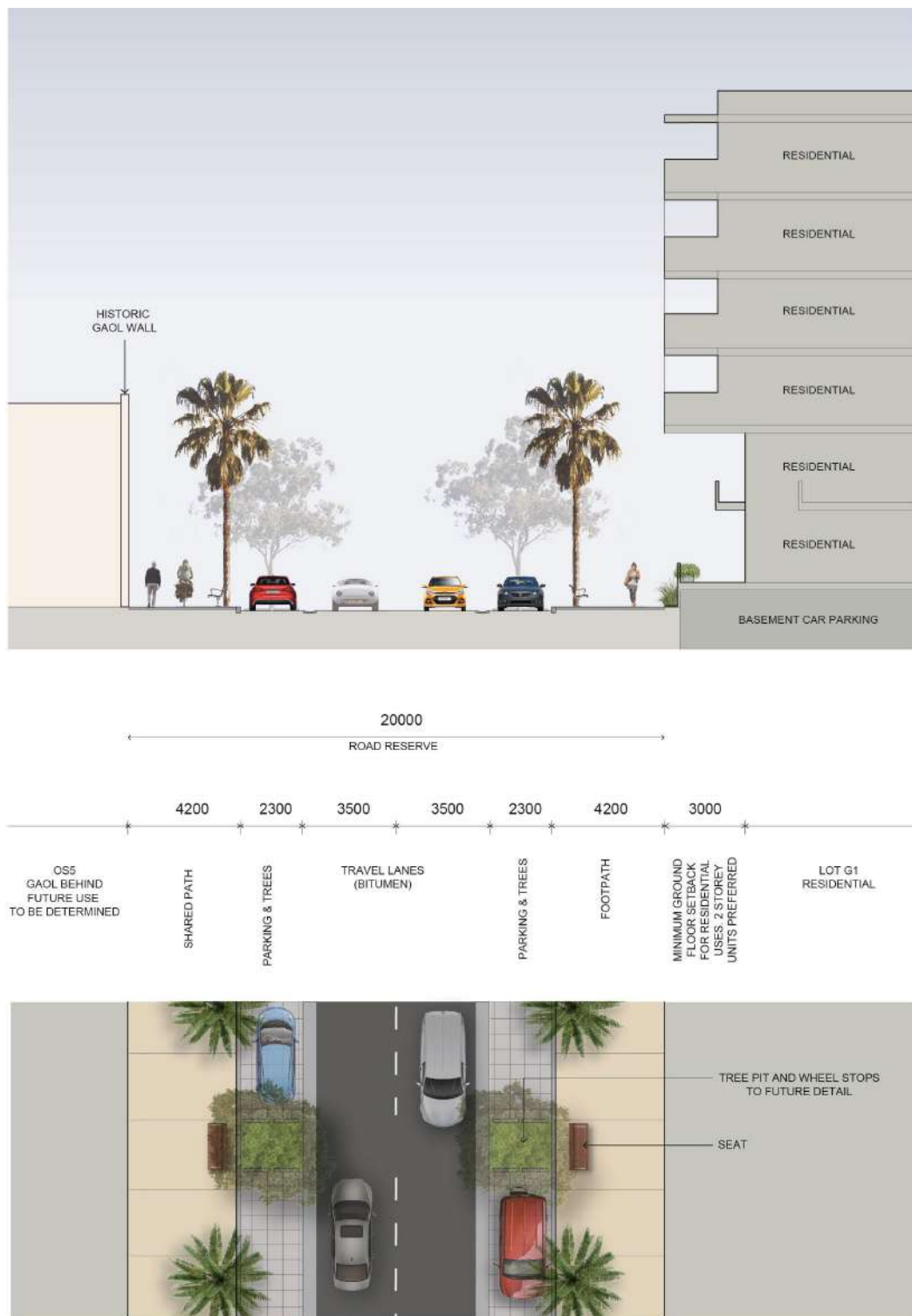
Figure 8.2.2.6.3 - Typical street section 3 – Dunlop Street
