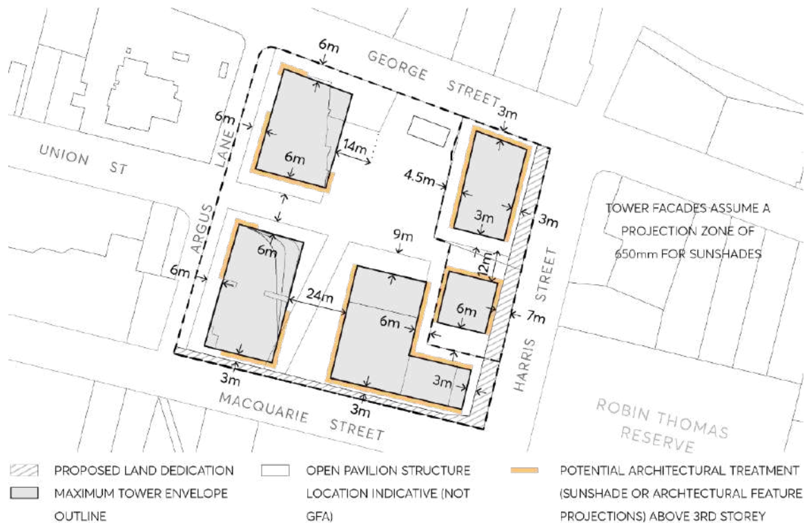
Figure 9.10.10.8 – Control diagram: Setbacks to towers above podium
