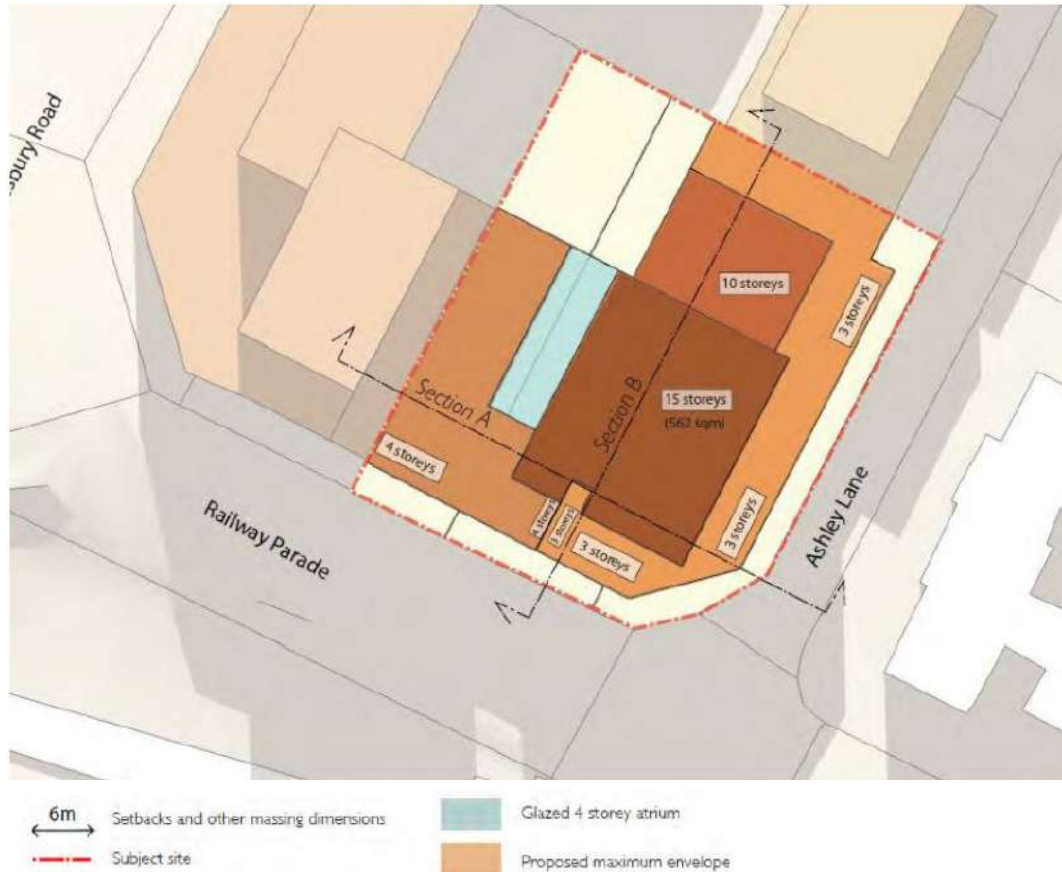
Figure 8.5.2.1.1 – Built form controls – Storeys
