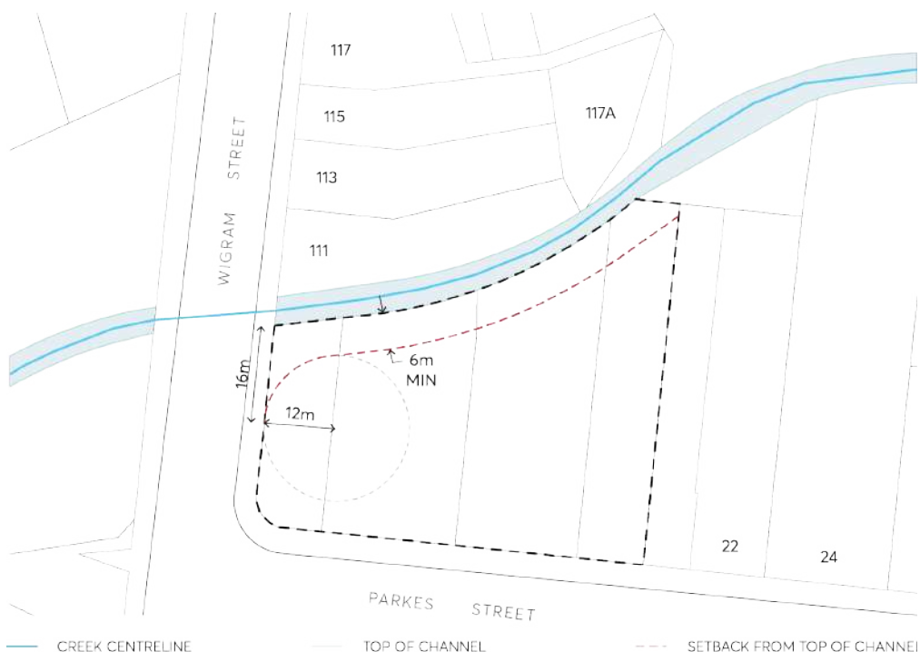
Figure 9.10.8.2 – Required floodway setbacks
