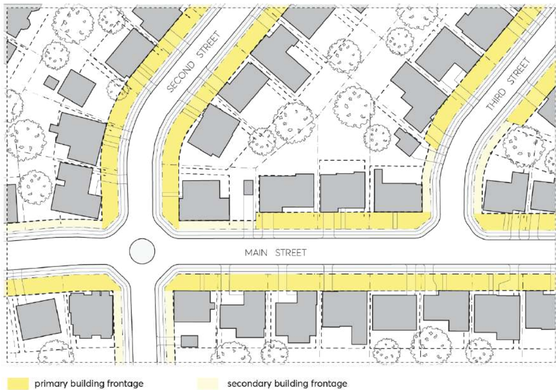
Figure 2.5.2 - Determining primary and secondary street frontages on infill lots
