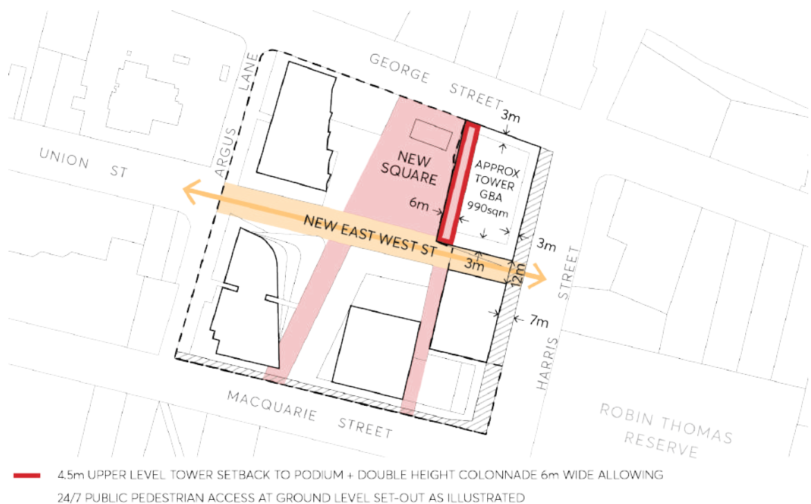
Figure 9.10.10.9 – Height of buildings in storeys and setbacks to towers over podium on former Albion Hotel Site
