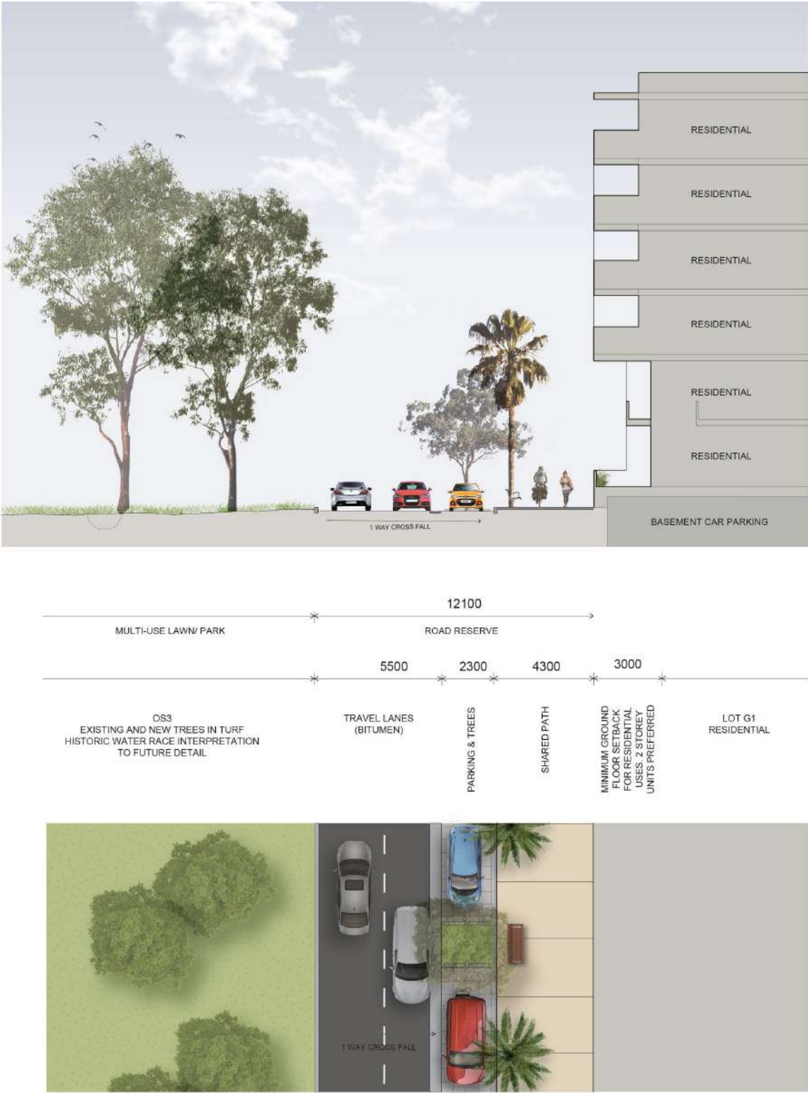
Figure 8.2.2.6.6 - Typical street section 6 – East Circuit (east)
