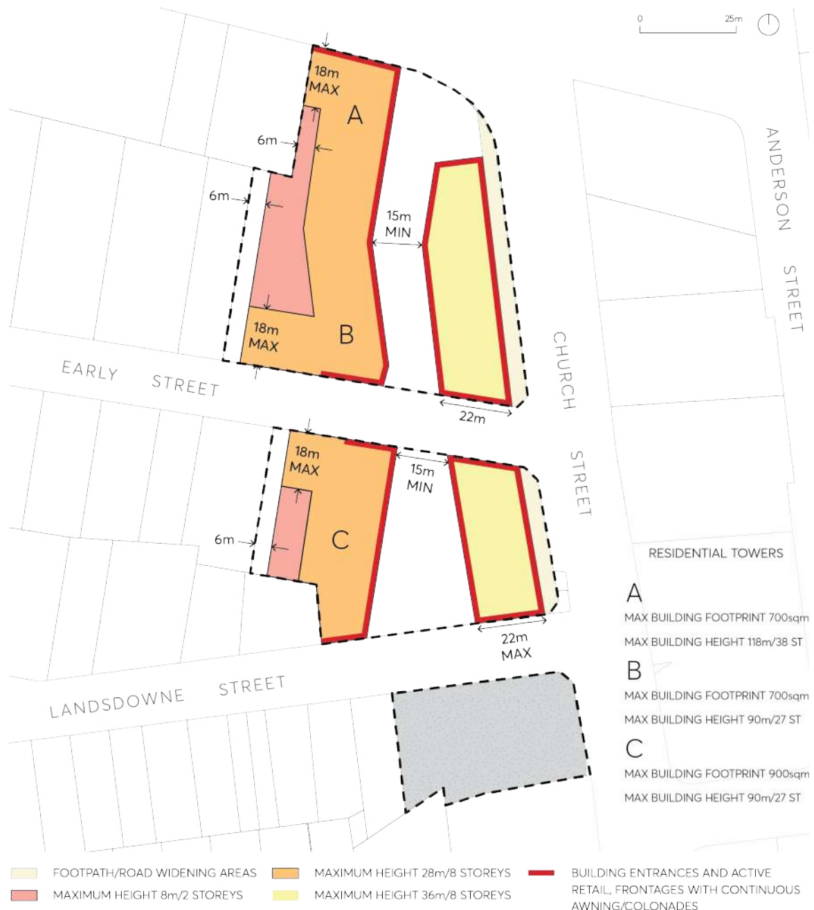
Figure 9.10.2.3 – Building Form Control Plan
