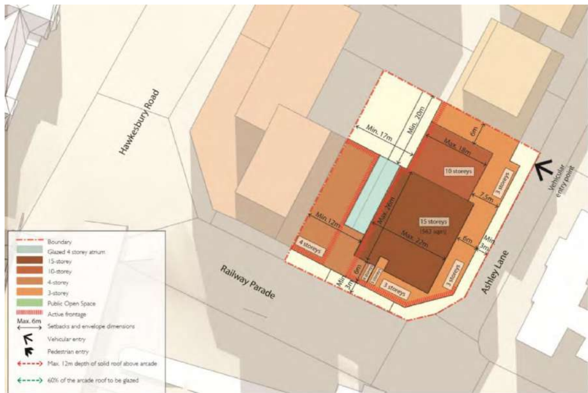
Figure 8.5.2.2.1 – Built form controls – Setbacks and building depths
