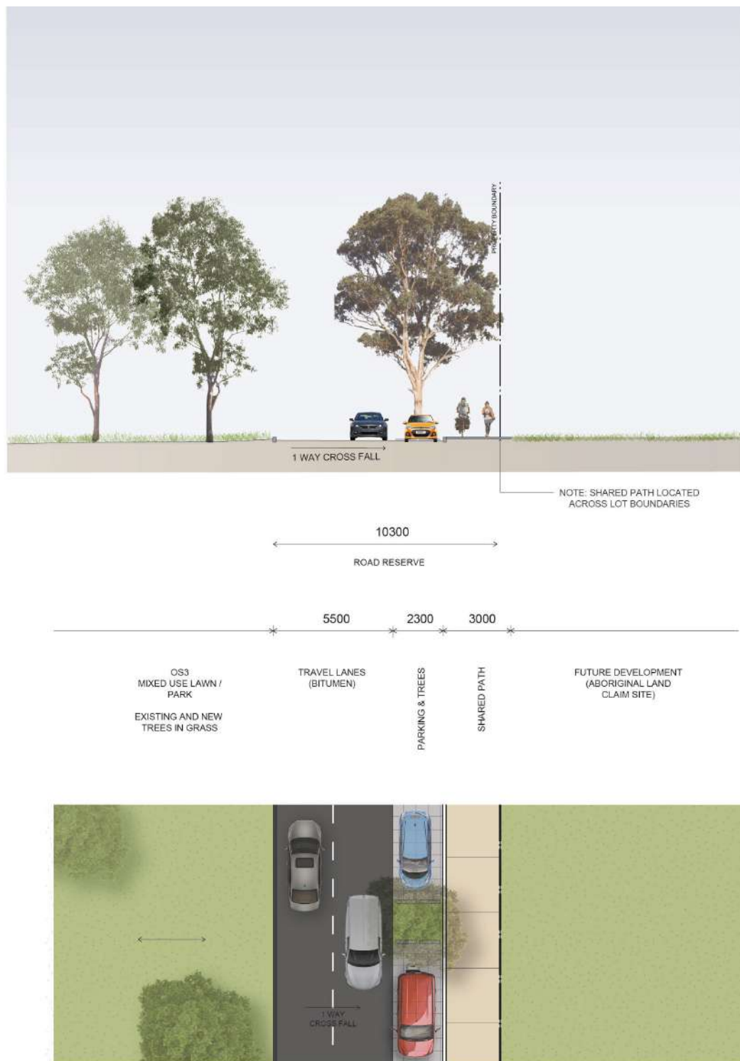
Figure 8.2.2.6.8 - Typical street section 8 – East Circuit (north)
