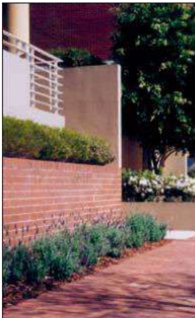
Combined wall/fencing materials with planting elements to soften the hard edge (Source: Residential Flat Design Code)
