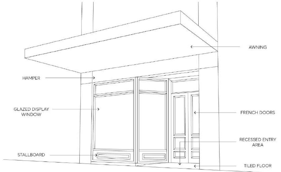
Figure 7.4.14 – Elements of a traditional early 20 th century shop front
