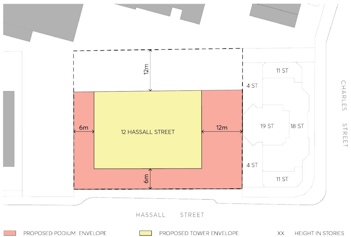
Figure 9.10.13.2 – Built form – setbacks and tower separations
