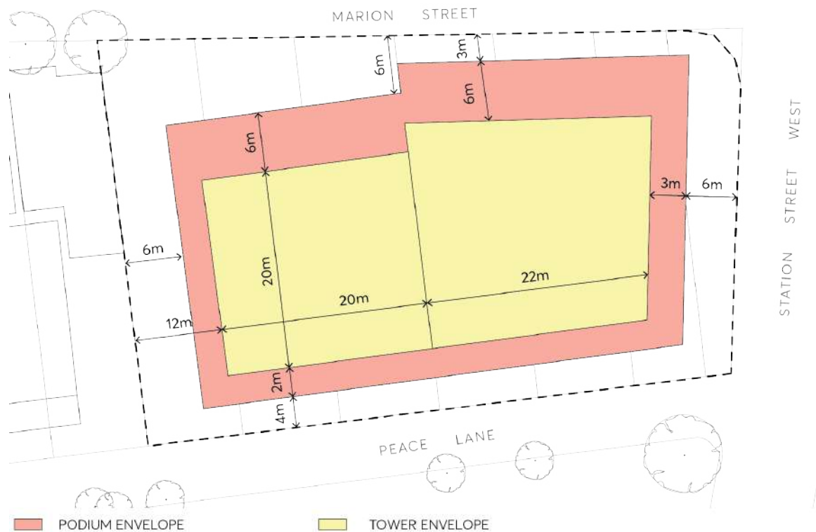
Figure 9.10.11.2 – Building alignment and setbacks
