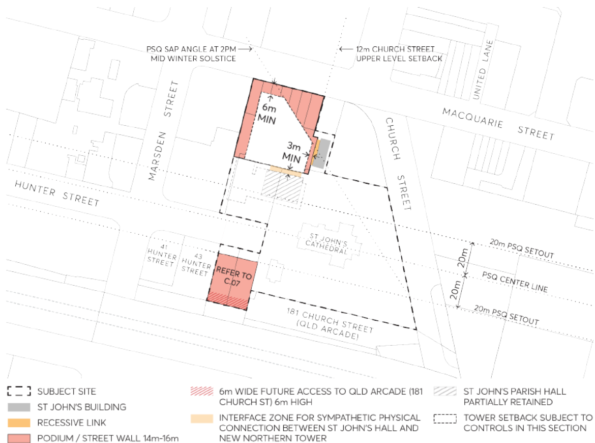
Figure 9.10.21.9 – Built Form set-out plan for Option B
