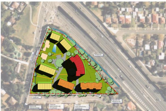
Figure 12 Shadow Diagram June 21 1200
